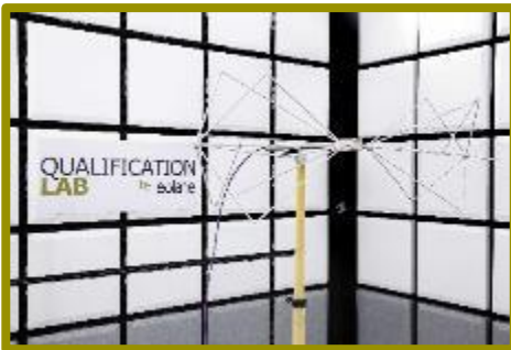
Anechoic Chamber Size 7m x 4m x 3,3m
