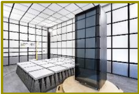
Anechoic Chamber Size 7m x 4m x 3,3m
