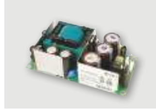
Medline 100 OFM100 Series 100W Open frame 2" x 4" Universal input 90-264VAC Low leakage 75uA EN55011/22 Class B Single output 12, 15, 18 or 24VDC
