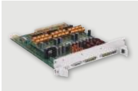
670W coreless technology DC/DC power supply, fully DSP-regulated converter for use in strong magnetic fields such as in MRI systems. 2.4 MHz switching frequency.
