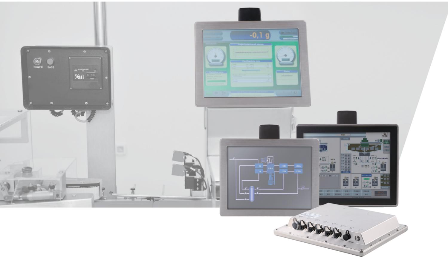
WP series Stainless steel Resistive/Multi-touch Panel PC is designed to meet the challenges in critical environments. It supports a wide operating temperature range from -20°C to 60°C and can withstand vibration. PC combined with a fully IP69K rated water/dust-proof enclosure and 6 x M12-type connectors, can resist ingress of high-temperature steam and pressure washing, well suited for food and chemical industry, as well as outdoor applications such as gas station or parking management system.
