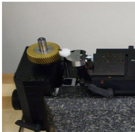
Clamping fixture for smallest gears
