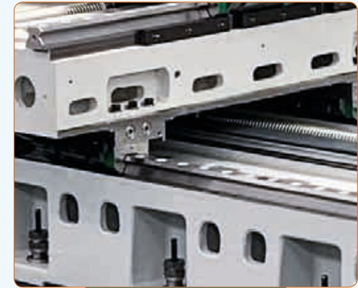
Cast iron structure
